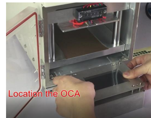
4. Locate oca and compress it on the rubber.
