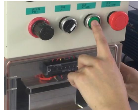
6. Press on the door and then start.
