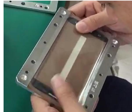
4. Locate glass and press the rubber bar.
