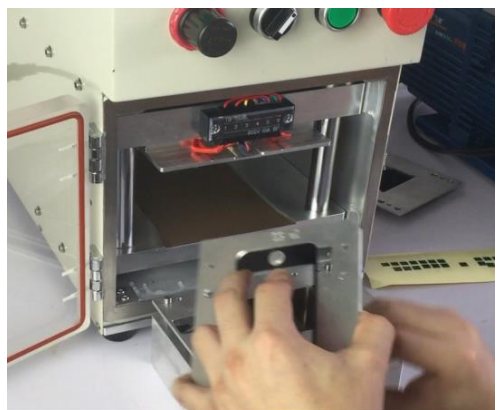
3. Direction downwards to place glass with oca.
