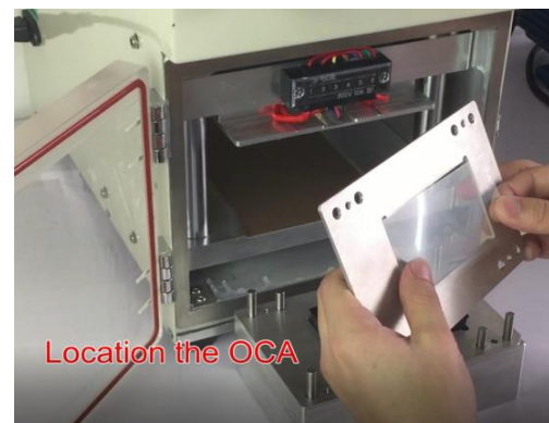
3. Use the oca mold piece to locate oca.
