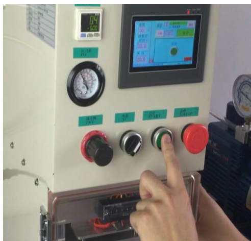
8. Press on the door and then start.
