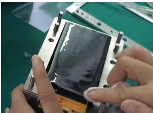
3. Clean the Lcd in one direction.
