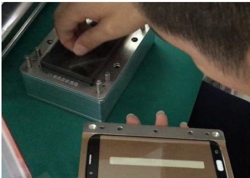
5. Tear protective film and place the glass mold top.
